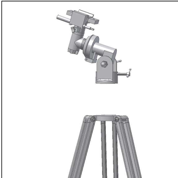
Figure 4. Place equatorial head on top of tripod.
