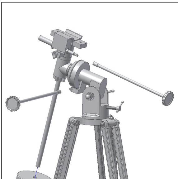
Figure 6. Fix Dec. and R.A. handles.
